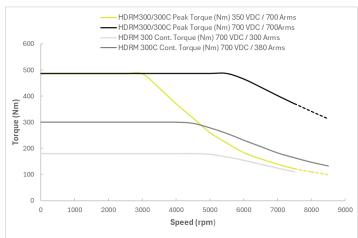
HDRM300 maximum speed 7.500rpm. HDRM300C maximum speed 8.400rpm.
